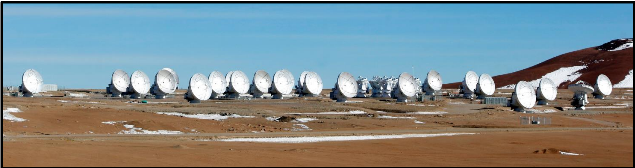
Figure 1: The Atacama Large Millimeter/submillimeter Array in Chile. The individual antennae work together as a single telescope. Credit: ALMA (ESO/NAOJ/NRAO), C. Padilla.
